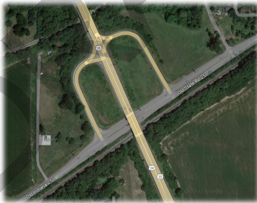
Figure 1: Low-Cost Interchange Example
